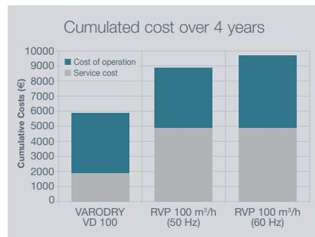
**Compared to an oil-sealed rotary vane pump, the VARODRY VD 100 saves > 650 EUR in operational costs per year!**
