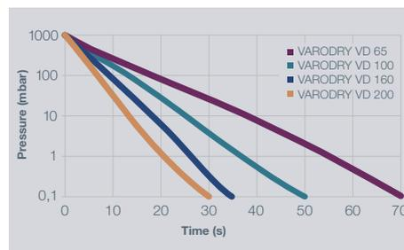
\*+/-10% tolerance; measurements at operation temperature for a 100l chamber with DN40 pipe and angle valve.
