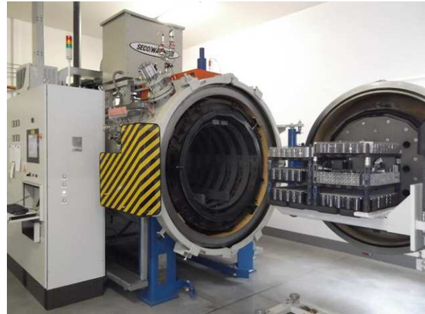
Fig. 2. Vector line, single-chamber, LPC, gas quenching vacuum furnace, up to 25 bar
