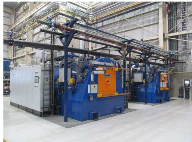
Fig. 3. CaseMaster Evolution line, three-chamber, preheating, LPC, oil quench, flow-through vacuum furnaces (semi-continuous)
