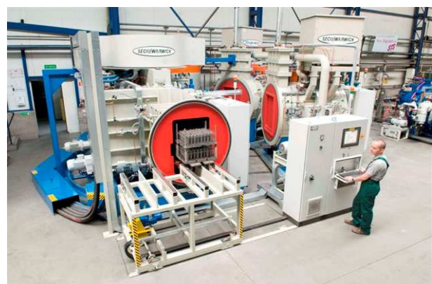
Fig. 4. A modular, multi-chamber, rotary system with LPC and 25 bar gas quenching for mass scale heat treatment
