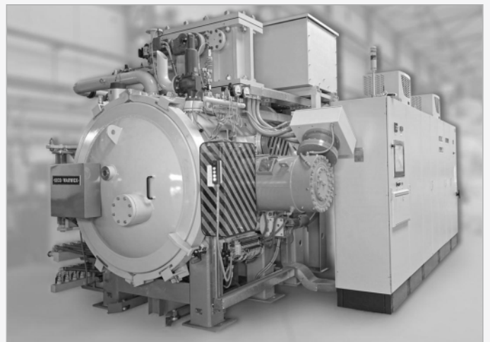
Case hardening CMe-D669-25 – double-chamber, LPC and 24 bar gas quenching
