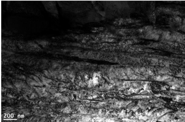
Figure 8. Microstructure of cast steel after isothermal quenching, TEM image
