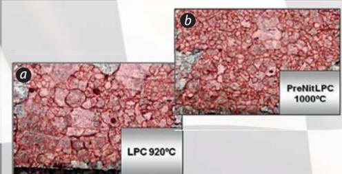
❷ Case structure of steel 16MnCr5 depending on the applied technology:
