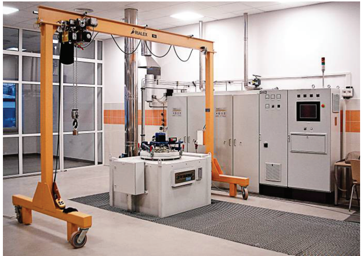
Fig. 13. Pit furnace of VRN type for gas nitriding using the ZeroFlow method.
