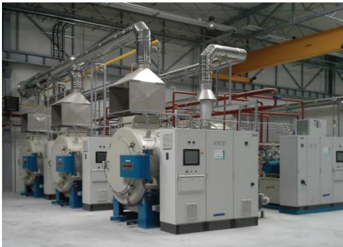
Fig. 12. Production line for gas nitriding with using the ZeroFlow method with HRN horizontal retort furnaces.
