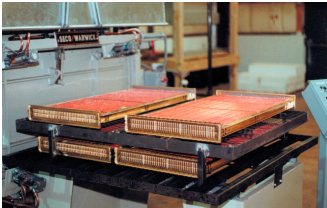
Double layer of radiators being brazed in a SECO/WARWICK CuproBraz® furnace.
