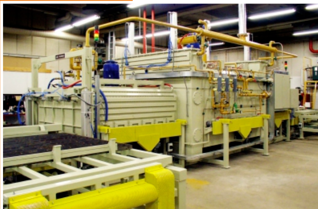
Three Chamber Semi-Continuous CuproBraz® Furnace.
