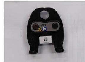
Parts made of 20MnCr5 steel are carburized to the layer of 0,5 mm, quenched and tempered in order to obtain a surface hardness in the range of 58-62 HRC. In the layer's structure, oxidation on the grains boundaries and emitting of carbides is unacceptable. Parts' mechanical fatigue is required counted in 20 000 working cycles (50 000 for type test).
