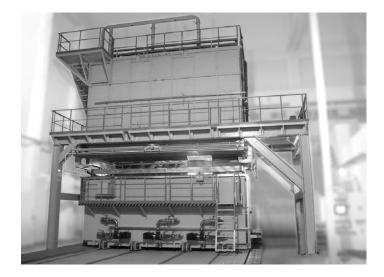
This innovative AMS compliant technology enables very fast and full load immersion as short as 5 seconds. As the VertiQuench name implies, the process provides very fast vertical quenching. The heat-treated material is dropped into water or polymer quenching tanks located directly under the furnace.
