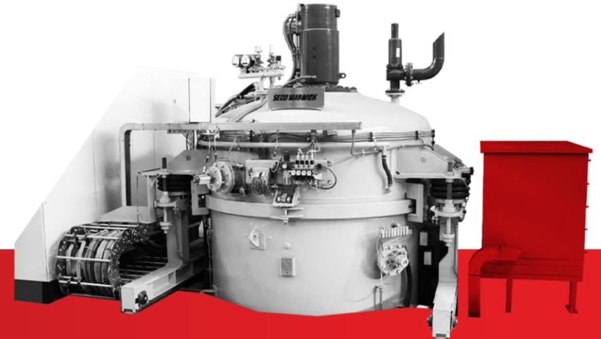
**Pit-LPC** shortens the carburizing process (2-3 times) by eliminating the need to prepare the process atmosphere. This significantly reduces energy and process gas costs. Additionally, the ability to replace up to three atmospheric furnaces with one vacuum solution reduces both investment and operating expenses.
