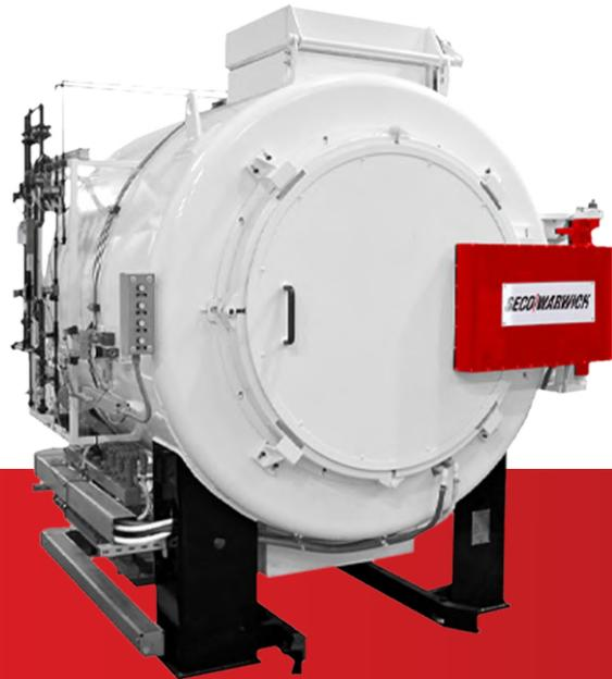
**ZeroFlow** - precise control of the nitriding potential lowers process costs and significantly improves the environmental impact of the process.
