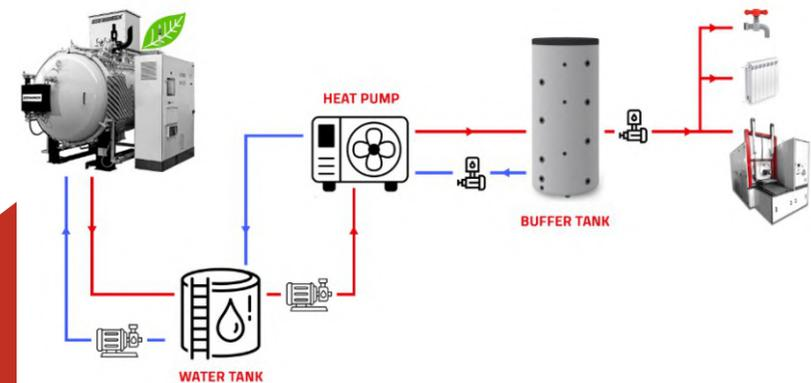
**Heat recovery** from an industrial furnace fully utilizes waste heat in other production processes.
