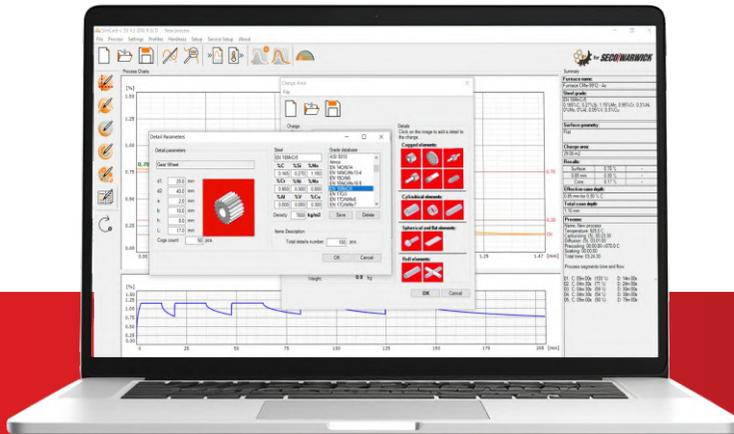
**SimVAC** optimizes the consumption of process gases by adjusting their amount to actual needs. Reducing gas losses and precise carburizing control reduces costs and increases energy efficiency.
