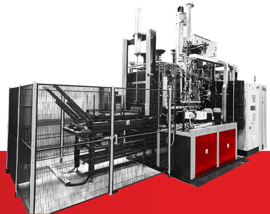
**Super IQ** combines the advantages of vacuum carburizing and traditional oil quenching, optimizing technological processes. The ability to work at higher temperatures accelerates production cycles, increasing plant efficiency and reducing operational costs.
