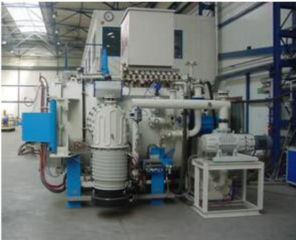
A control manifold provides all necessary ports for vacuum and pressure gauging. A further valve port is provided for connection to the helium leak detector.
