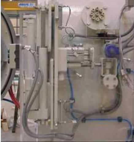
A hinged front door provides access for work loading, periodic cleanup and system maintenance. A lip seal located in a groove in the cover flange seals the flange-to-flange contact between the furnace chamber body and front cover, on closure of the vessel. Door clamp operated by linear motor allows positive pressure operations.
