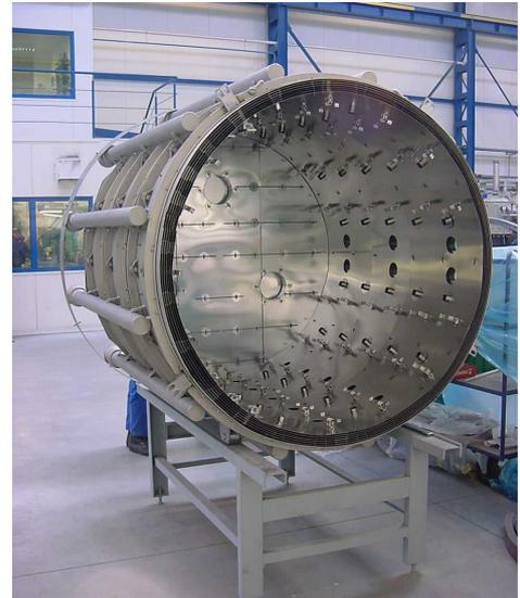
Each power terminal is directly coupled to one of the copper power feedthroughs in the space between the hot zone and vacuum vessel. The sidewall elements are arranged in few circuits, bottom-to-top, for optimum temperature uniformity; individual slats are connected by molybdenum nuts and bolts to facilitate replacement in the event of damage. A minimum number of parts are used.
