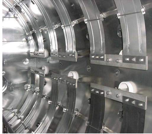
The elements and power terminals are supported from water-cooled feed-throughs on the wall of the cylindrical heating chamber and are accessible from the hot face side of the thermal insulation assembly. The hot part of the power terminal is fabricated from molybdenum and is electrically isolated by a ceramic sleeve where it passes through the heat shield (this ceramic is protected from the rigors of the cooling cycle) and is protected against metallization during brazing operation.
