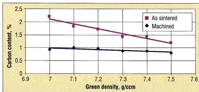
**Fig. 3.** %C on the carburized surface showing dependence on density – SECO/WARWICK pulse/pause process
