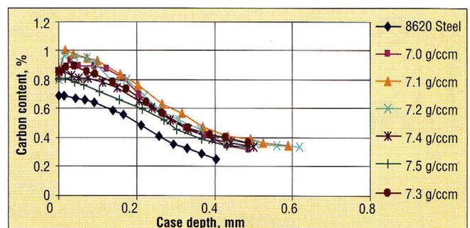
Fig. 2. Carbon distribution showing dependence on density (machined surfaces) - SECO/WARWICK pulse/pause process
