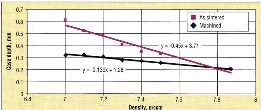
**Fig. 7. Case depth at 0.5% C showing dependence on density for machined and as-sintered surfaces – Hayes pulse-pump process**
