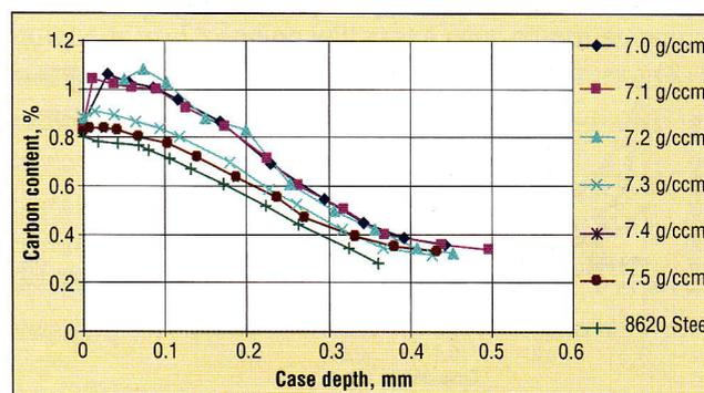
**Fig. 6.** Carbon distribution showing dependence on density (machined surface) – Hayes pulse-pump process
