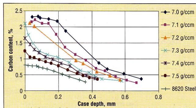
**Fig. 5.** Carbon distribution showing dependence on density (as-sintered surfaces) – Hayes pulse-pump process
