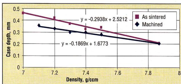
**Fig. 4.** Case depth at 0.5% C showing dependence on density for machined and as-sintered surfaces – SECO/WARWICK pulse/pause process
