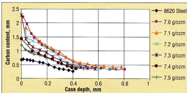
Fig. 1. Carbon distribution showing dependence on density (as-sintered surfaces) - SECO/WARWICK pulse/pause process
