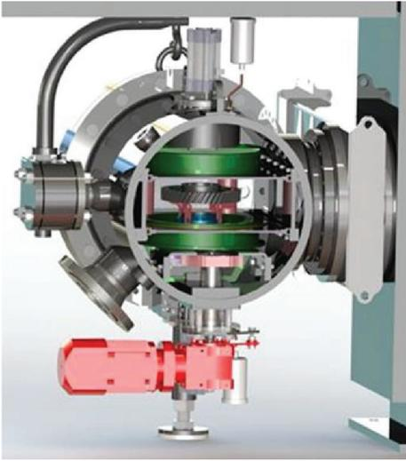
Figure 8: 4D quenching chamber for HP&GQ
