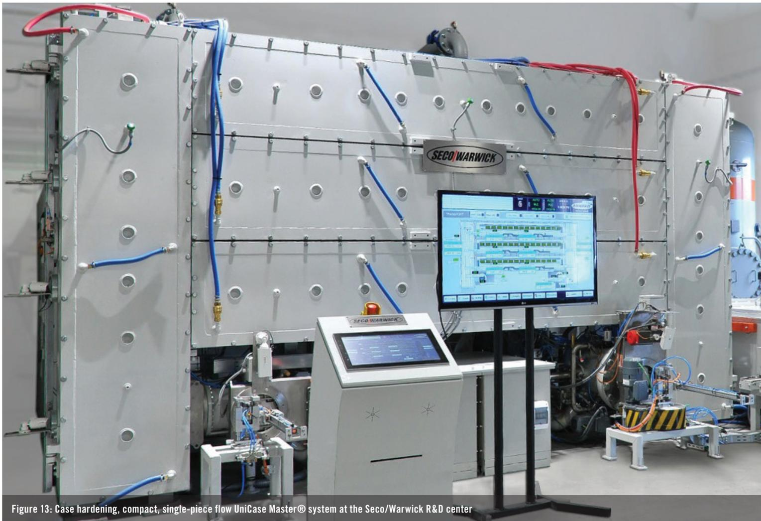
Figure 13: Case hardening, compact, single-piece flow UniCase Master® system at the Seco/Warwick R&D center
