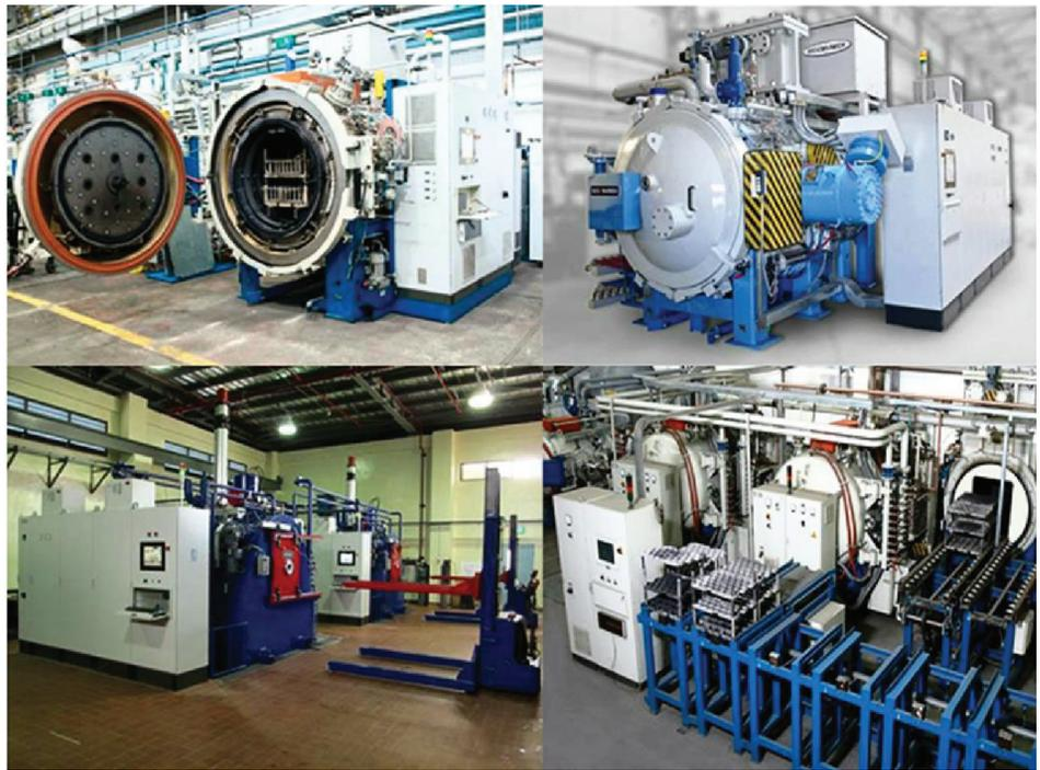
**Figure 4: Vacuum furnaces for case hardening (top: single- and double-chamber HPGQ; bottom: double-chamber oil quench and multi-chamber HPGQ)**
