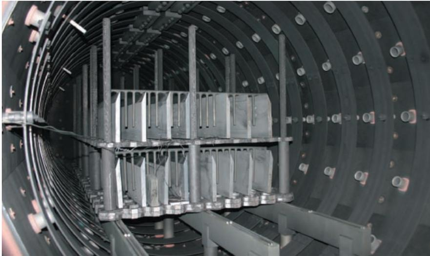
Fig. 3 — HPQ furnace with 36 × 32 × 140 in. work chamber designed for thermal treatment of knives (cutters) made of AISI S5 steel.
