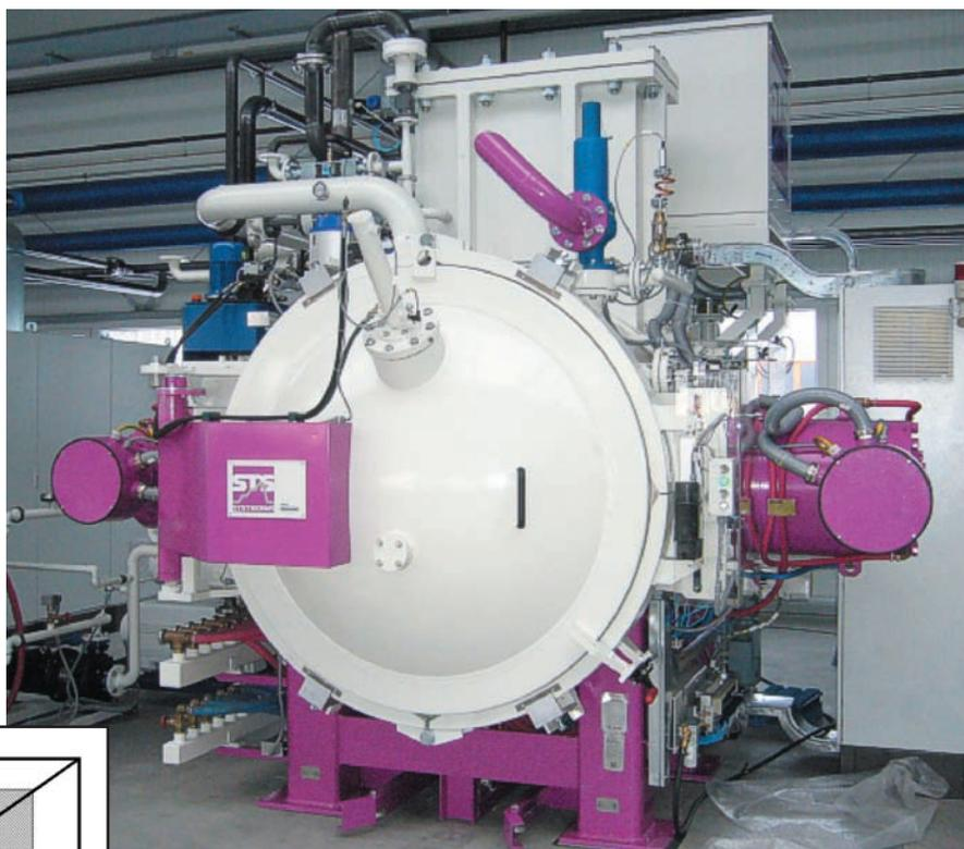
Fig. 9 - Double-chamber 24 x 24 x 36 in. furnace with 20-bar quenching.
