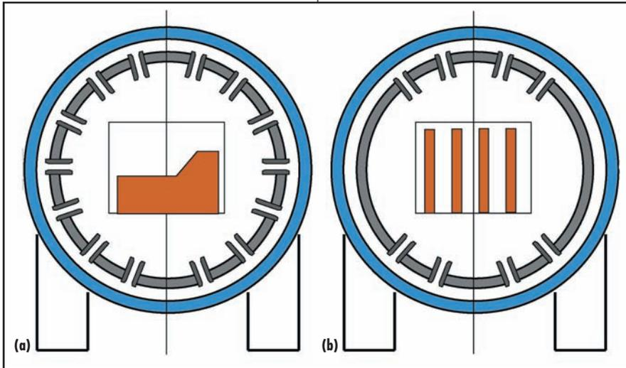
Fig. 2 — Radial gas flow (a), and axial gas flow (b).
