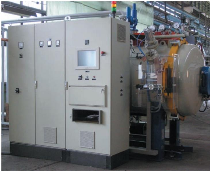
Fig. 7 — HPQ furnace with 16 × 16 × 24 in. work chamber.
