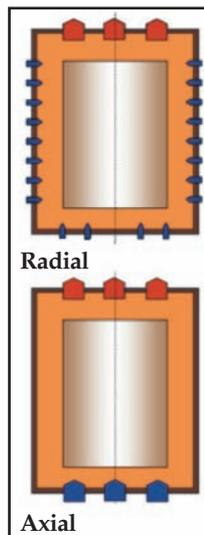
fect on quenching rates (Fig. 6). Furthermore, in furnaces with larger heating chambers, achieving the parameters mentioned above is more difficult, while in furnaces with smaller heating chambers (e.g., 16 × 16 × 24 in.), more dynamic quenching conditions can be achieved. Quenching rates measured in the core of test bars achieved in a 24 × 24 × 36 in. furnace at 700°C (1290°F), which are suitable for hardening of certain grades of carburizing steels, are shown below
