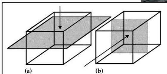
Fig. 10 - Flow area through useful space (a) axial, (b) radial.
