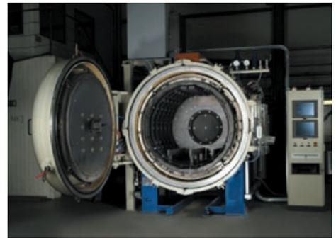
Fig. 1 -- HPQ furnace with axial/radial quenching system.
