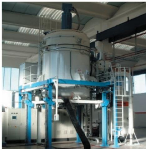
Fig. 5 — Elevator furnace (72 in. diam. × 72 in. high) with axial/radial quenching.
