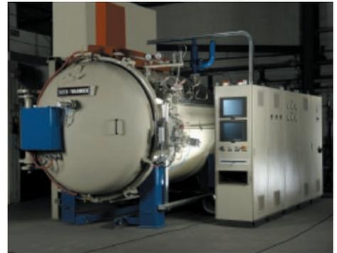
Typical HPQ furnace with 16-bar gas quenching.
