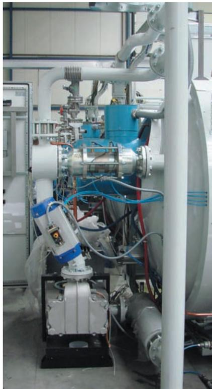
Fig. 8 - Pumping system for 25 bar hydrogen.
