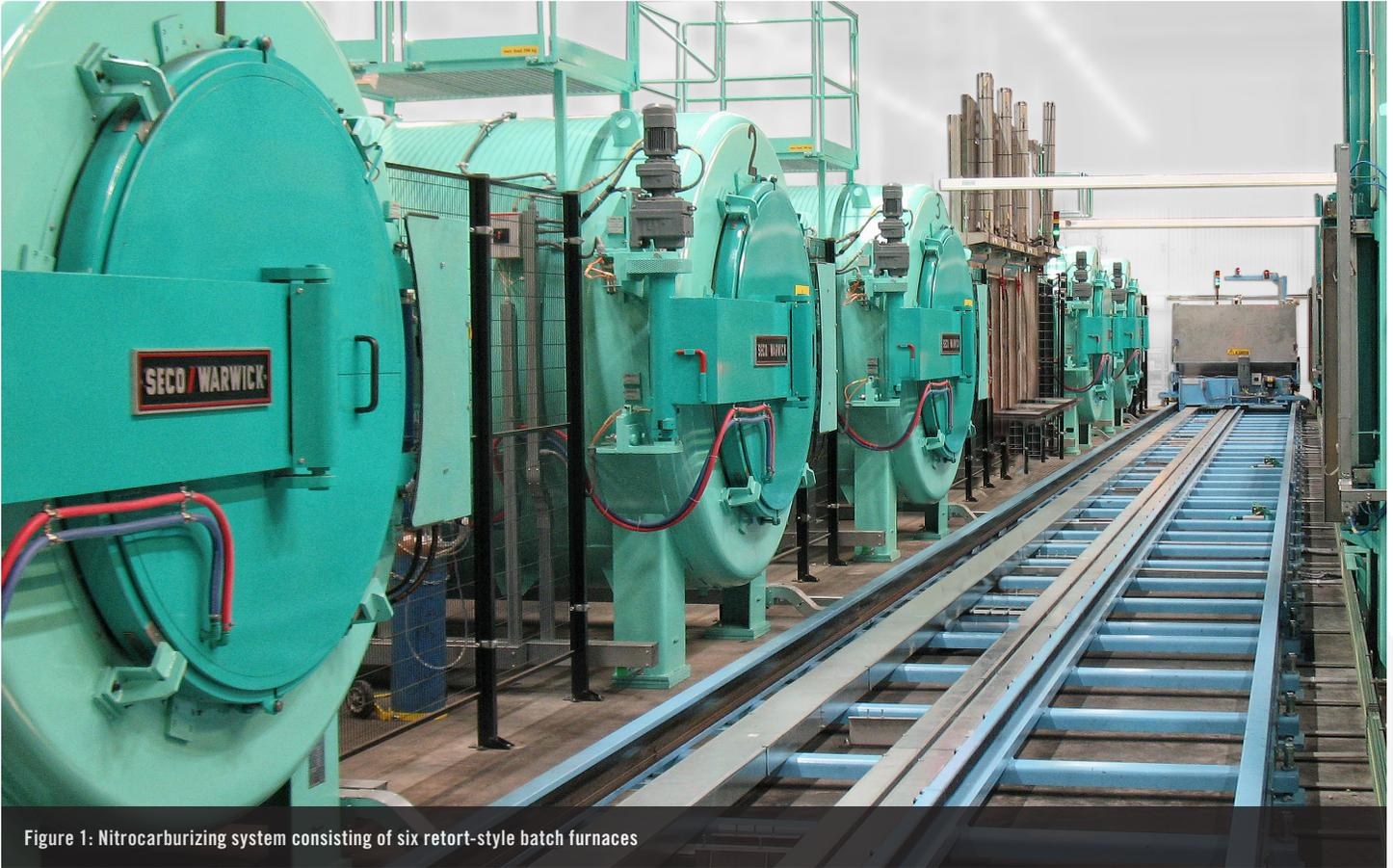
Figure 1: Nitrocarburizing system consisting of six retort-style batch furnaces
