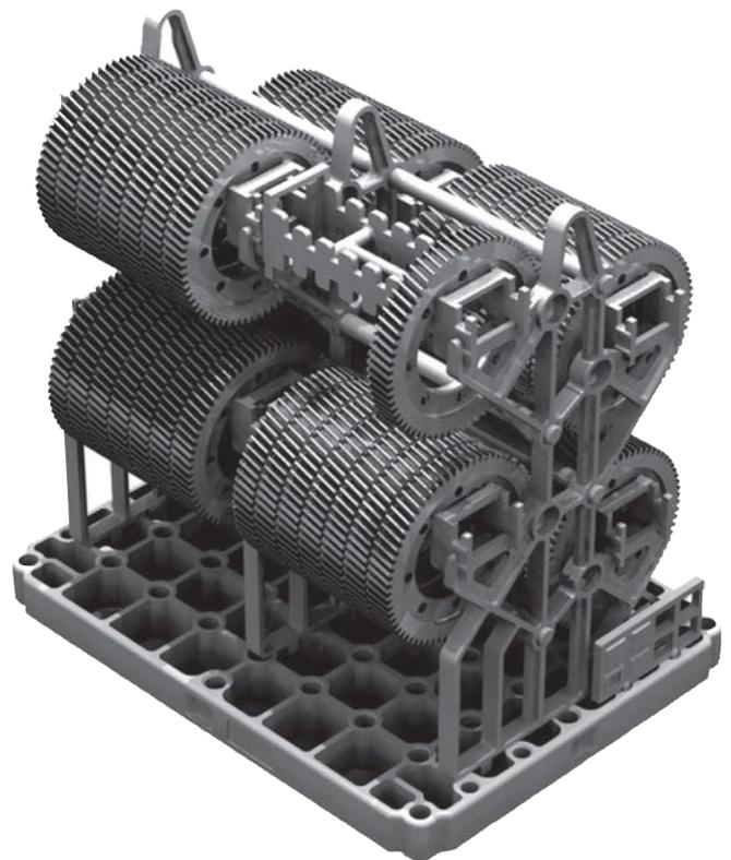
Figure 4: Gears for ferritic nitrocarburizing
