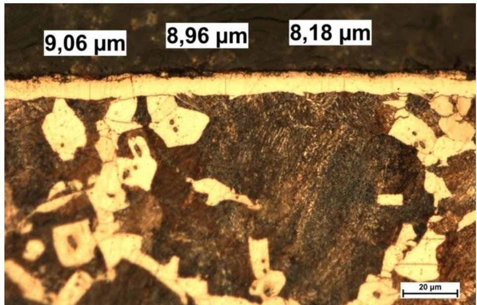
Figure 7: Microstructure of case in nitrocarburized 4120 alloy steel
