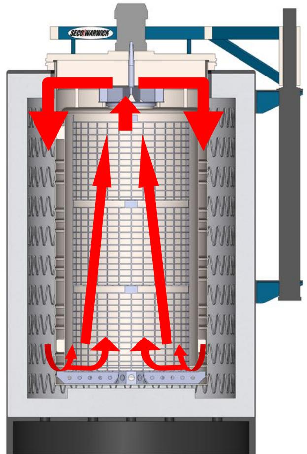
Figure 3: Schematic of pit-type retort nitriding showing gas convection flows
