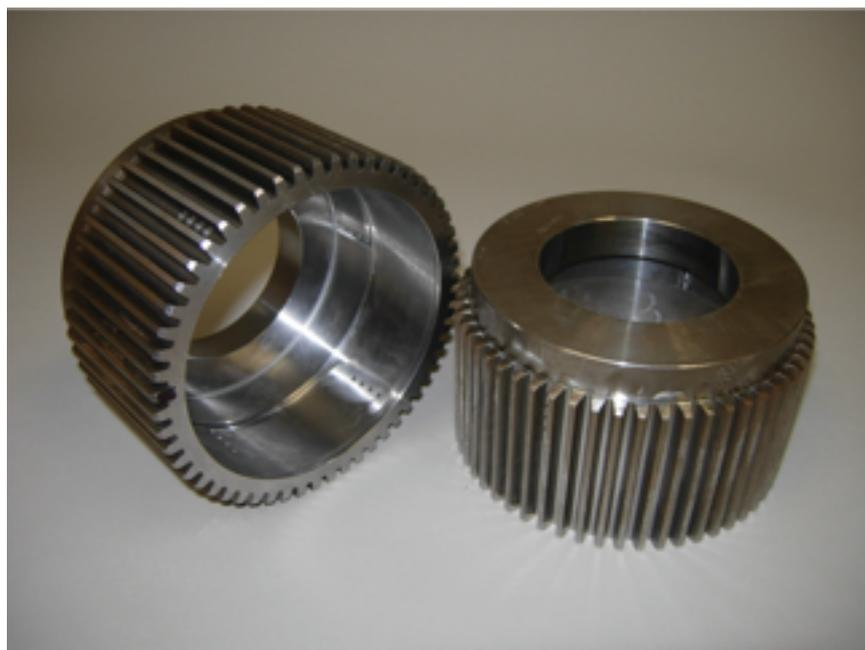
Figure 5 | 150 mm (6") clutch hub; test gear type "C"
