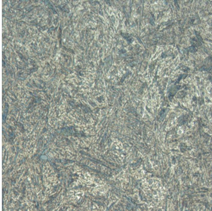
Figure No. 15 | Clutch gear "C", gear tooth mid-radius, AC + OPQ, (1250X, 2% Nital)
