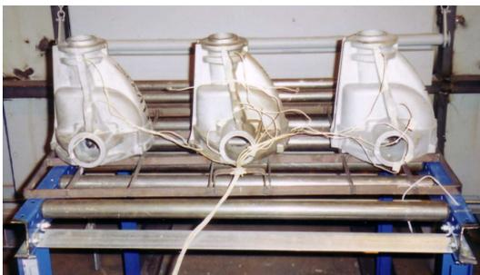
Fig. 5 Test load of Castings
