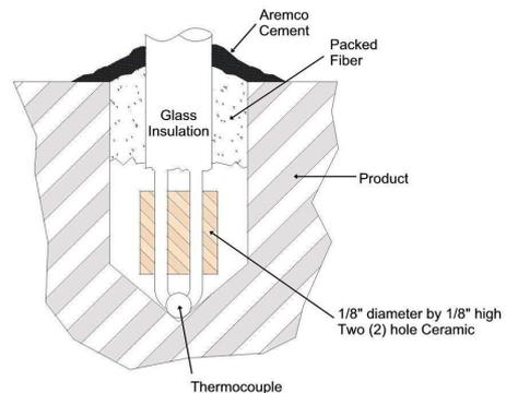
Fig. 4 Thermocouple Configuration
