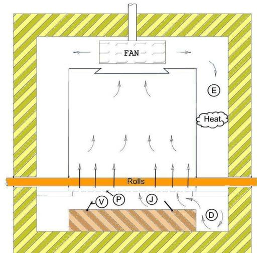
Fig. 1 Mass Flow – Jet Impingement Furnace
