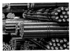
from 40–130 mm can be very flexibly rolled from a small number of feed cross-sections. The hydraulic adjustment of the rolls that permits roll gap control under load allows dimensional deviations due to temperature or material behaviour to be equalized. A complete workshop for roll changing and adjustment in the cassettes, including an optical setting gage, also forms part of the SMS group scope of supply.
