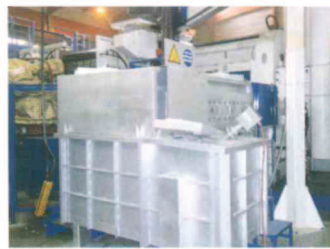
A heater with mobile station used during maintenance means 2 hours are gained per furnace monthly.
