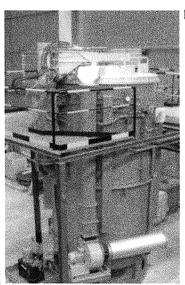
Dorssers Inc. manufactures dies with a wide range of specifications depending on production requirements, quality needs and the type of ingredient to be pelletized. The pellet dies are large diameter, hardened steel dies with a multitude of holes gundrilled for compressing various feed stocks. The environment is harsh, so exact heat treating is a must. The two electric
